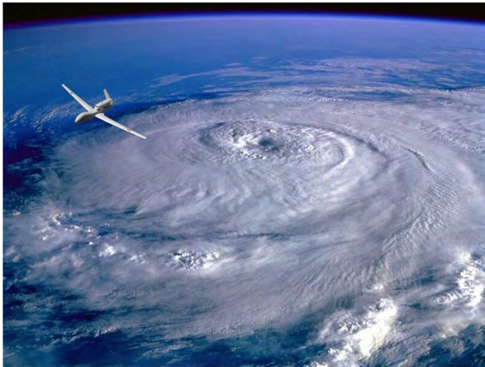
Figure 9. Unmanned drones, Global Hawks can over-fly hurricanes at altitudes greater than 60,000 feet with flight durations of up to 28 hours.
